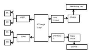
We are basically making an agricultural robot which will perform the operation like sowing the seeds, ploughing then covering the soil again and then sprinkling water as well.
